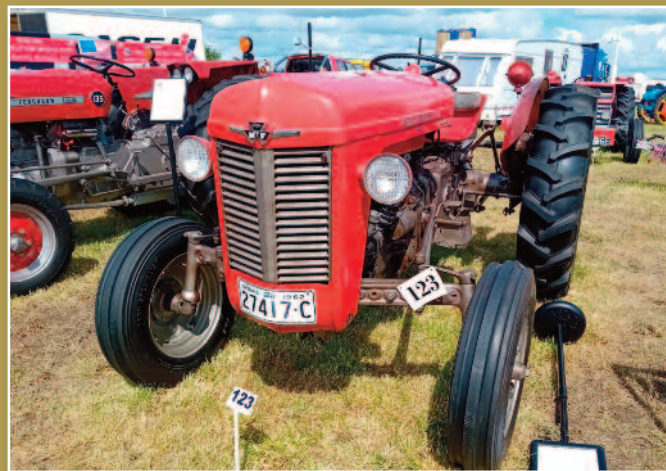
An American spec MF35 multipower, with a 3 cylinder Perkins petrol powered engine.
