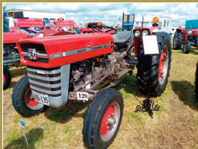
MF135 powered by a Perkins 3 cylinder petrol engine. Imported from Canada in 2022. Spent its working life in Ontario.
